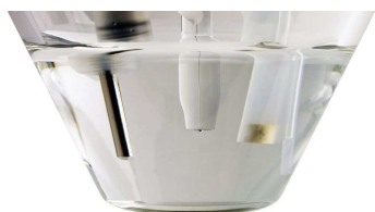
The Metrohm 3 electrode system. (the real physical diameter of the mercury drop is typically between 0.3 mm and 0.4 mm; the size is adjustable in certain narrow limits).
